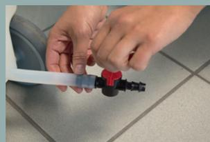
Drain the fresh and waste water tanks into a shower tray or a ground siphon.
