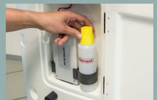
Open the waste water tank valve. Fill the disinfectant tank with water & BFR 4.0 disinfectant. Start the automatic disinfection device of the complete waste water circuit until the tank is empty.
